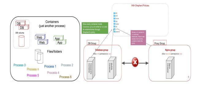
This diagram shows how Shepherd is integrated with Intel's CIT to ensure integrity at rest and run-time.
